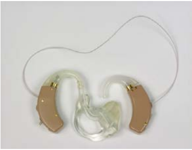
Figure 10 The photo shows two hearing aids connected by a wire and one hearing aid has an earmold. Contralateral Routing of Signals (CROS) takes sound from the deaf ear and transmit to the normal hearing ear with better hearing.
